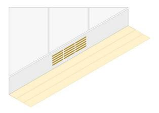
Venting slots of any shape, size or design can be cut in kick plate boards.
